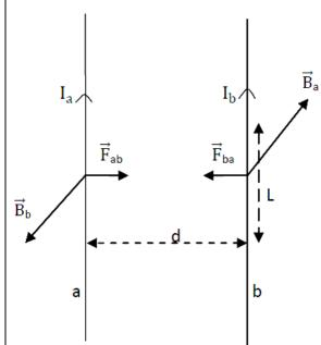
Labelled diagram (F<sub>ab</sub> and B<sub>b</sub> are not necessary in the figure)
