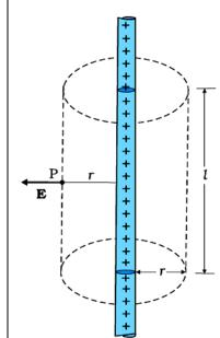
The electric field is everywhere radial, **flux through the two ends** of the cylindrical Gaussian surface is zero.
